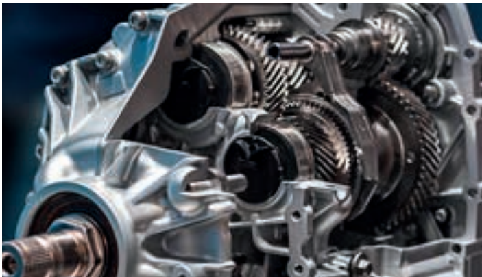
Gears hardened under vacuum
