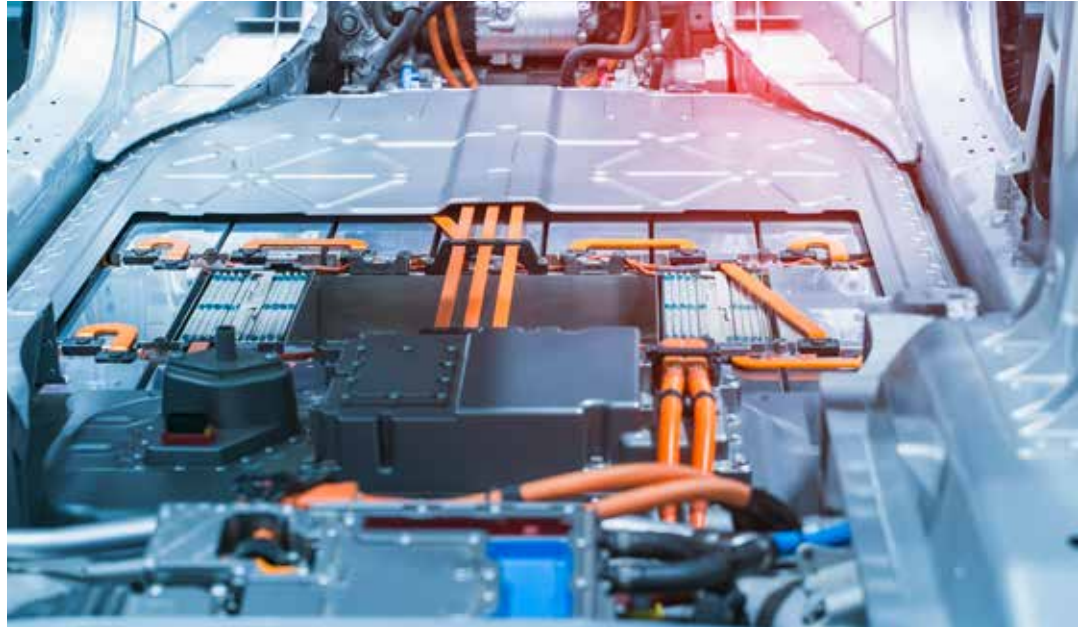
Battery pack with cooling system
