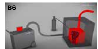
Integral test of helium filled parts in vacuum
