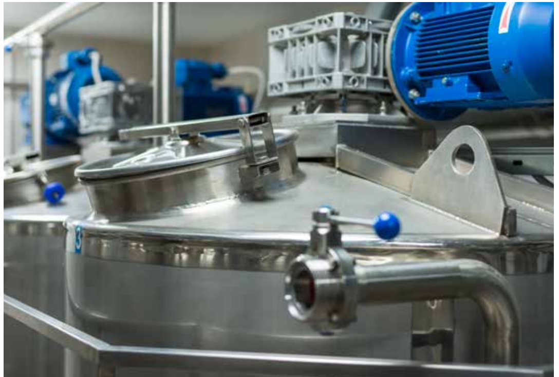
Mixing of the slurry under vacuum
