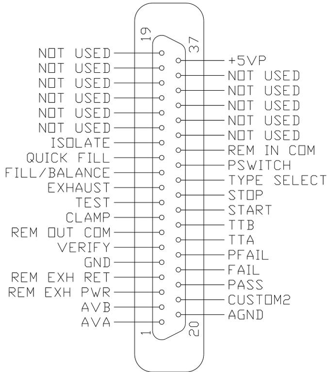
**Figure 3.2.2 – Standard Remote I/O Pin Connector**
