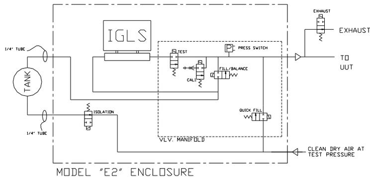
**Figure 3.1.1 - Pneumatic Connection**
