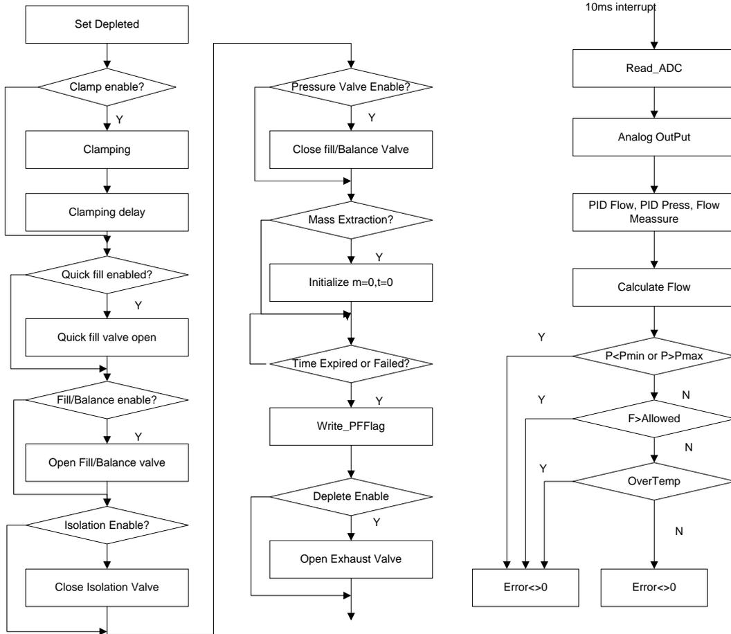
**Figure F.2 Mass extraction test control algorithm**
