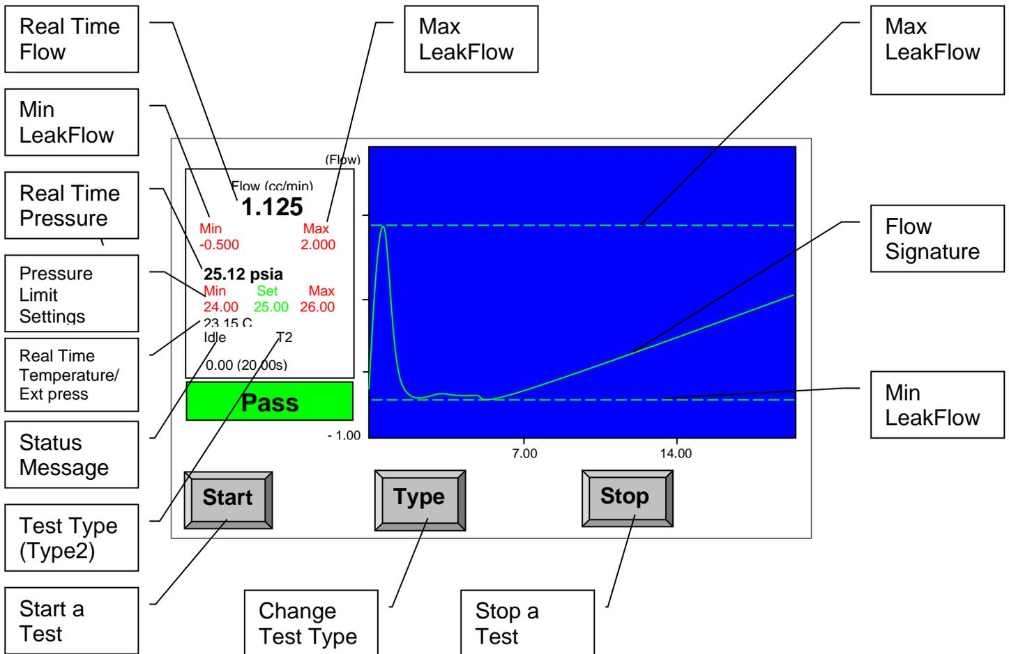
Figure 5.2 - Model "E2" or "VE2" LCD Elements
