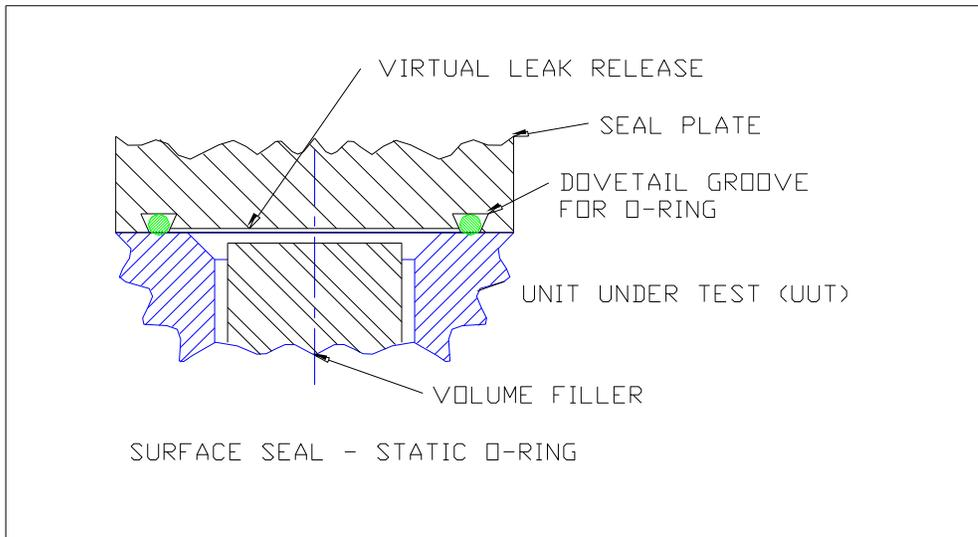
**Figure 3.4.1: Surface seal design with static o-ring.**
